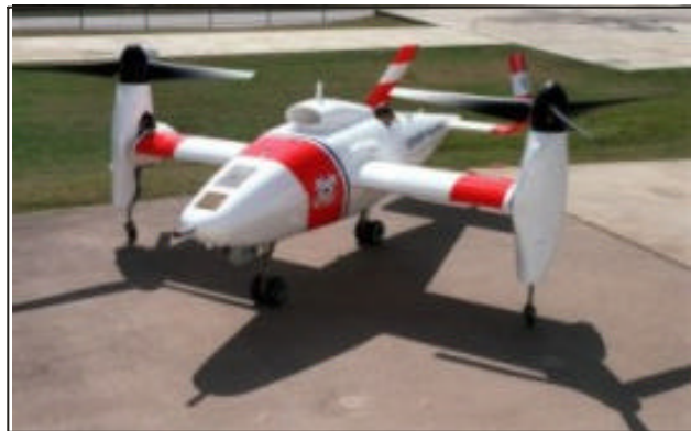
A contender for the US Marines is Bell's tilt-rotor, seen here in a fullscale prototype
